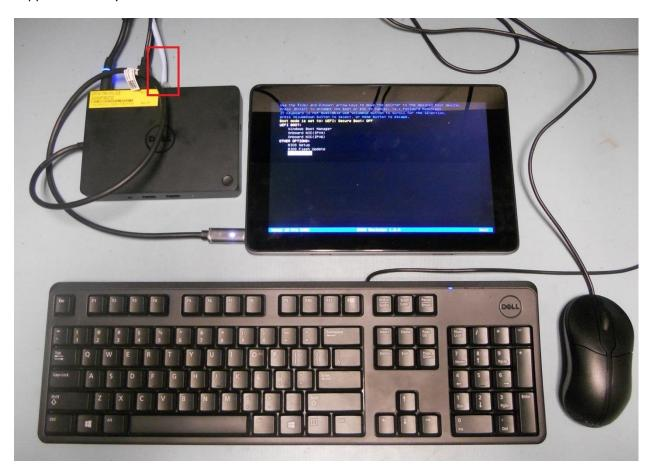
As an example of Latitude 5175/5179 boot up system with Ethernet connection to the WD15 docking, as soon as the Dell splash screen is displayed, press the F12 to bring up the one-time boot selection menu.
